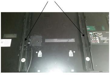
STEP SIX - LIFT THE TV ONTO THE MOUNTING BRACK ON THE STAND - MAKE SURE BOTH SETS OF FINGERS ON BOTH SIDES ARE ON CORRECTLY
