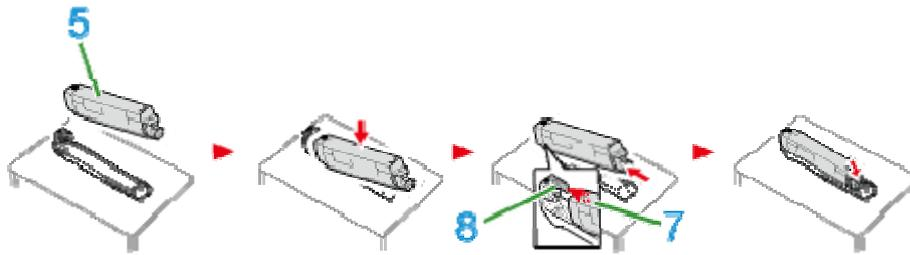
13. Turn the blue lever (6) of the toner cartridge backward until its top align on the
