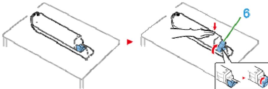
14. Check the label color of the new image drum and place the drum into the machine.
