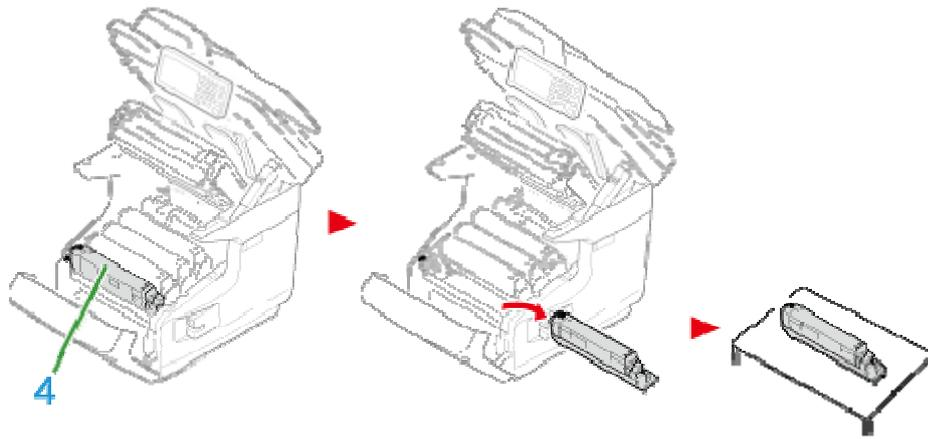
7. Turn the blue lever (6) of the toner cartridge toward you until its top align on the
