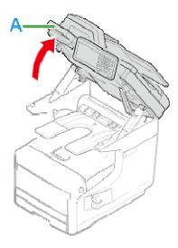
2. Insert your finger into the lever (B) on the right side of the machine and pull the front cover open lever (1) to open the front cover (2) forward.
