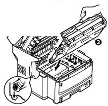
**10.** Turn the two fasteners (1) 90° to the right until they lock. This will secure the belt unit in place.
