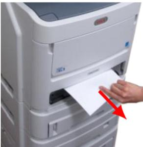
NOTE: Ensure all paper is undamaged, stacked properly and the paper guides are properly positioned against the edges of the paper stack
