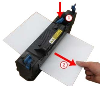
6. Holding the handle; insert the fuser unit back into position
