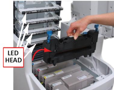
NOTE: Make sure the fuser unit does not hit the LED head
