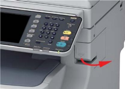
2. Pull out the cartridge and remove the jammed staple
