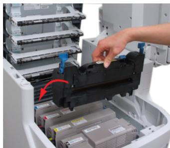
7. Push the blue lock lever (both sides) in the direction of the arrow toward the back of the machine to lock the fuser unit
