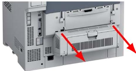
6. Lift the cover up (1) and remove the jammed paper (2)
